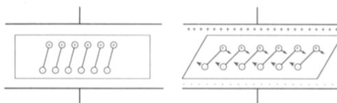
**Figure 1.** Schematic representation of the converse piezoelectric effect for shear motion. The electric field induces reorientation of the dipoles of the acentric material, resulting in a lattice strain and shear deformation of the material. Direction of shear is dependent upon the applied potential while the extent of shear strain depends on the magnitude of the applied potential.
