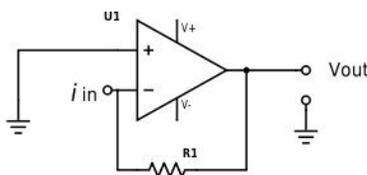
**Figure 2.** The current-to-voltage amplifier is used to amplify a small amount of current into a voltage that can be easily measured. The circuit obeys Ohm's law, so that the product of the input
