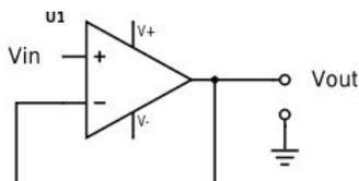
**Figure 1.** The voltage follower is the simplest op amp circuit made by connecting the inverting input and output pins of the op amp with a wire. This circuit is often used as a “buffer” to avoid impedance mismatches between voltage sources and measurement equipment or other parts of the circuit.
