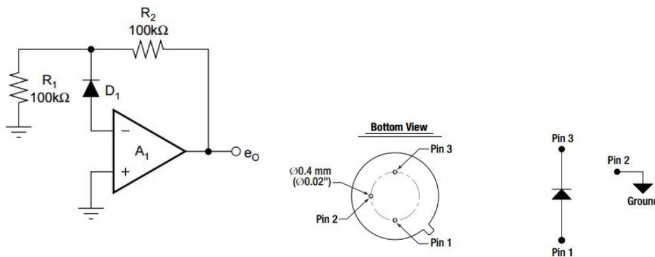
Figure 3. The current-to-voltage amplifier with the photodiode in the circuit (left) and the pin diagram for the photodiode (right).
